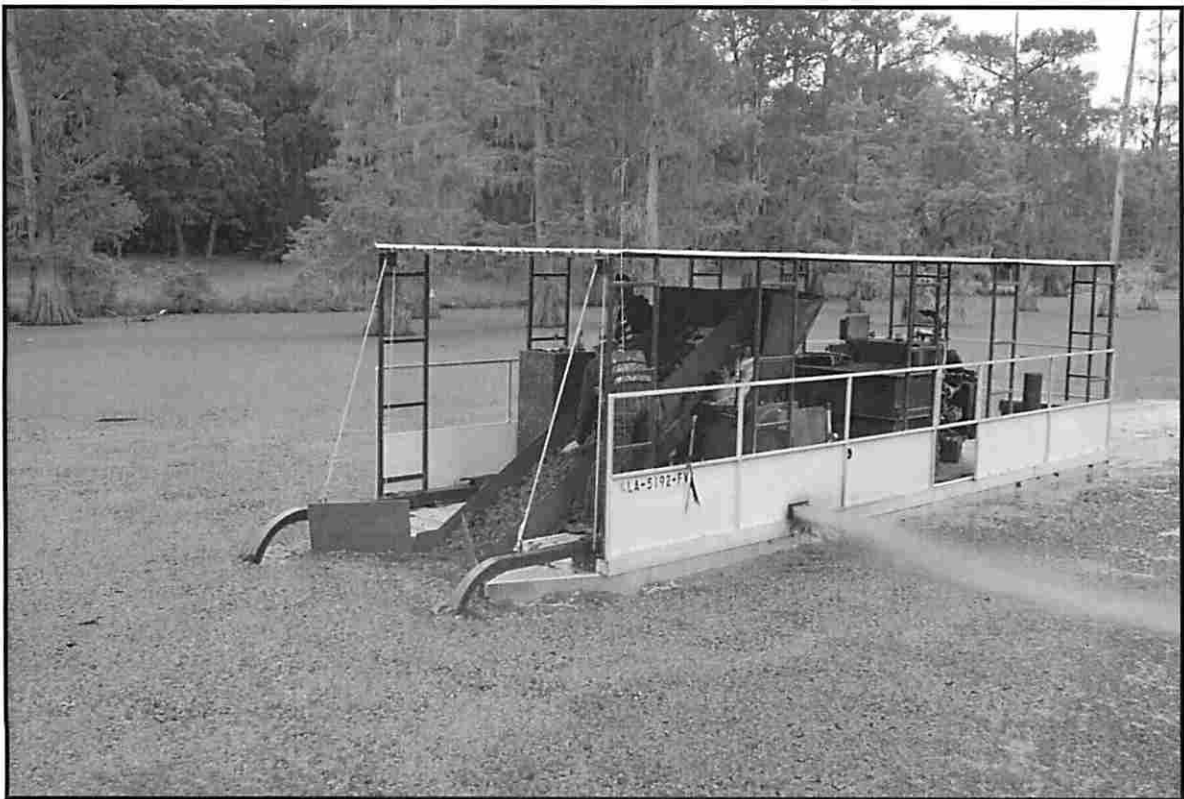
Figure 1. The WaterMower uses a conveyor belt on the front of the boat to transport the plant material from the water surface into a grinding machine. After the plants pass through the grinder, they are deposited from a chute on the side of the boat and back into the water. April 26, 2013.
